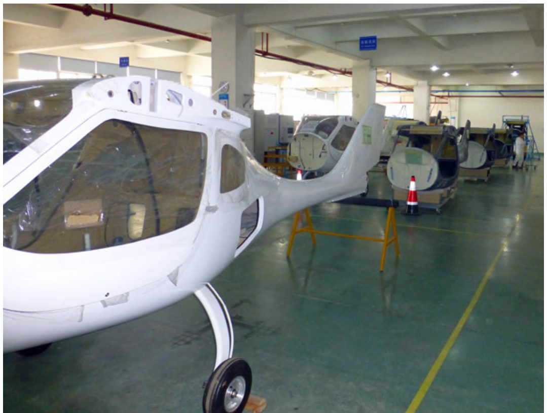
AeroJones CTLS models in final assembly production line.
