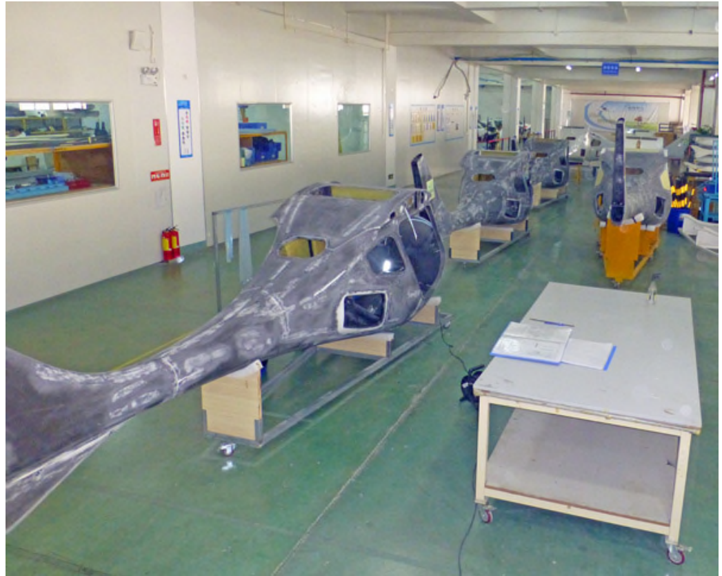
AeroJones' production line show CTLS Light-Sport Aircraft in carbon fiber.
