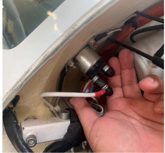
correct installation of starter solenoid
