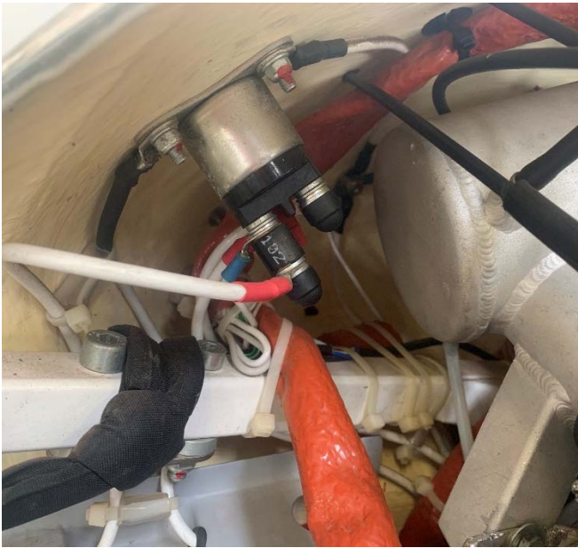
correct installation of starter solenoid
