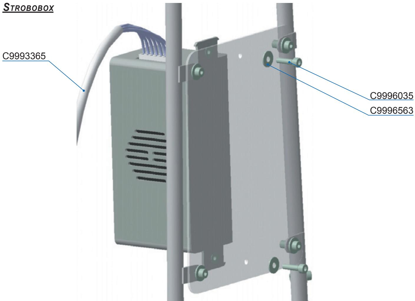
**Strobobox, StroboLight Quick Connection, Underfin Light, Wing Light**
