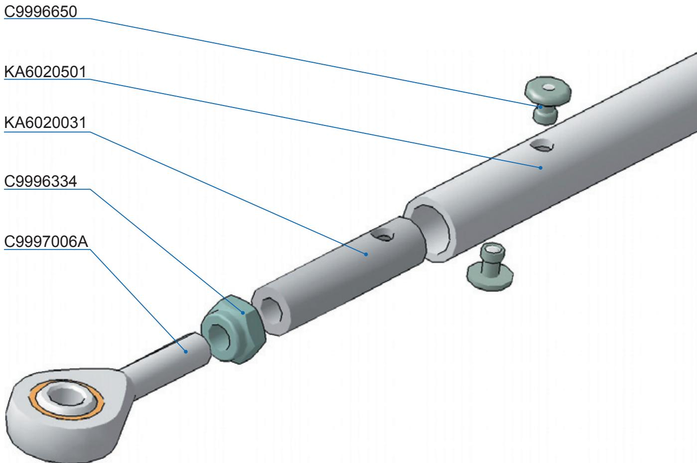
**KA6062000 – AILERON TRIM MECHANISM MOUNTING**
