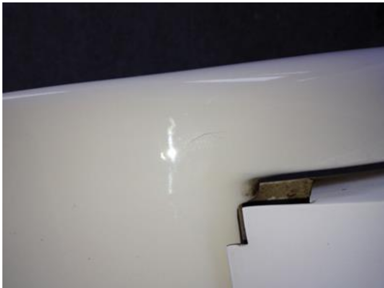
superficial crack in paintwork
