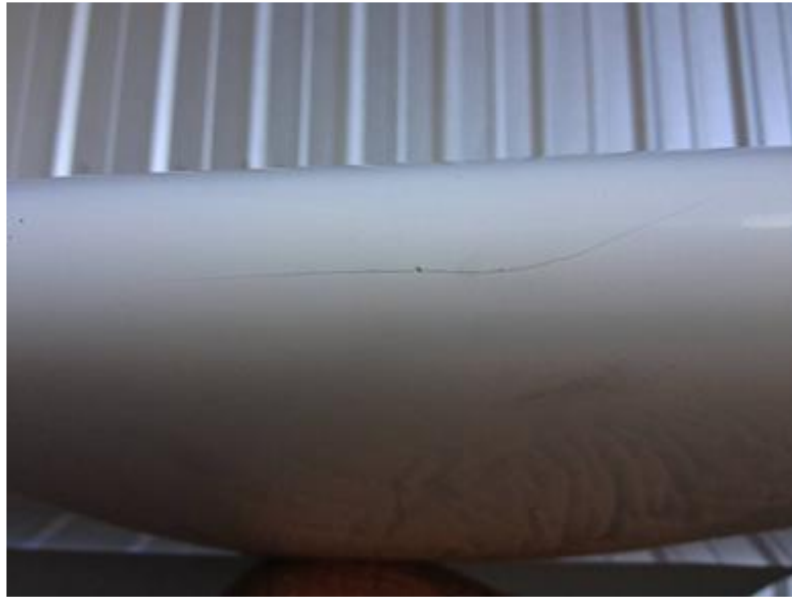
superficial crack in elevator leading edge
